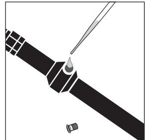
Fill the sensor shaft completely with KOH,
