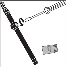
Unscrew the lock plug from the refill opening
