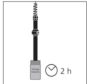
Before first use: store the sensor in the storage flask (filled with deionised water) for 2 hours
