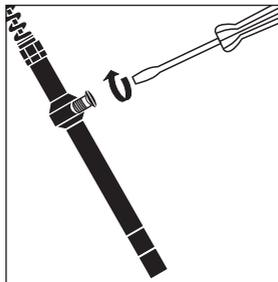
Screw the refill opening tight with the lock plug
